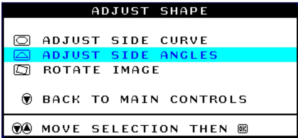
4) Press the
