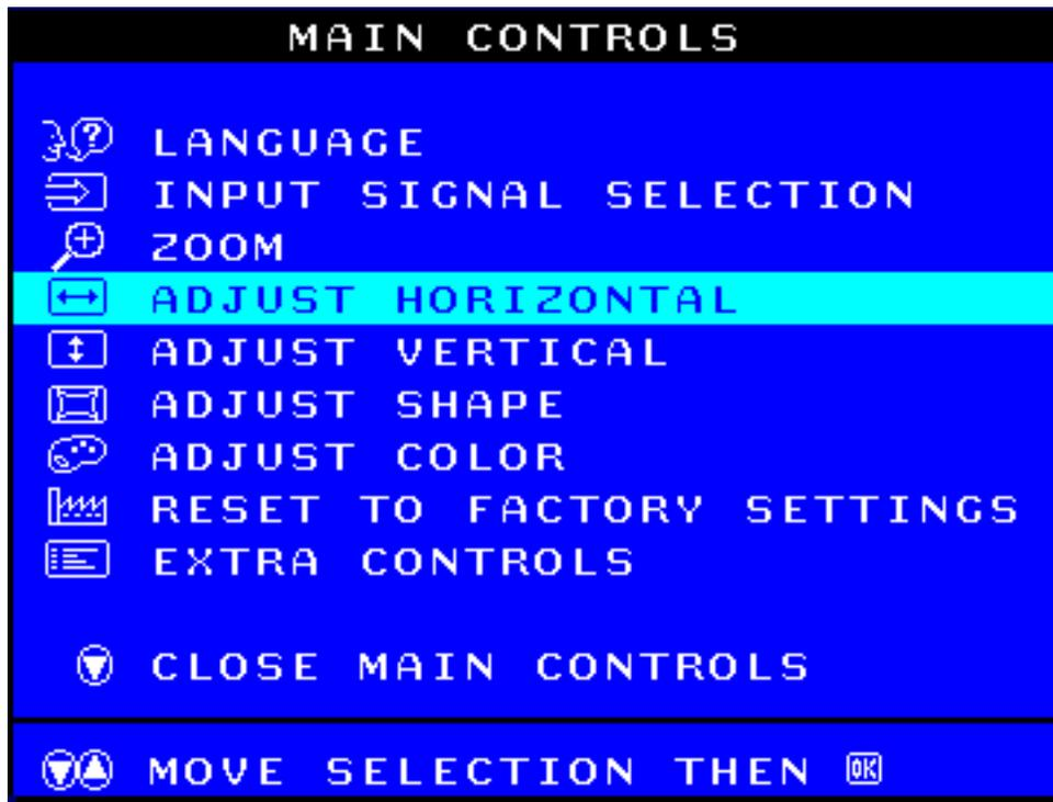
3) Press the
