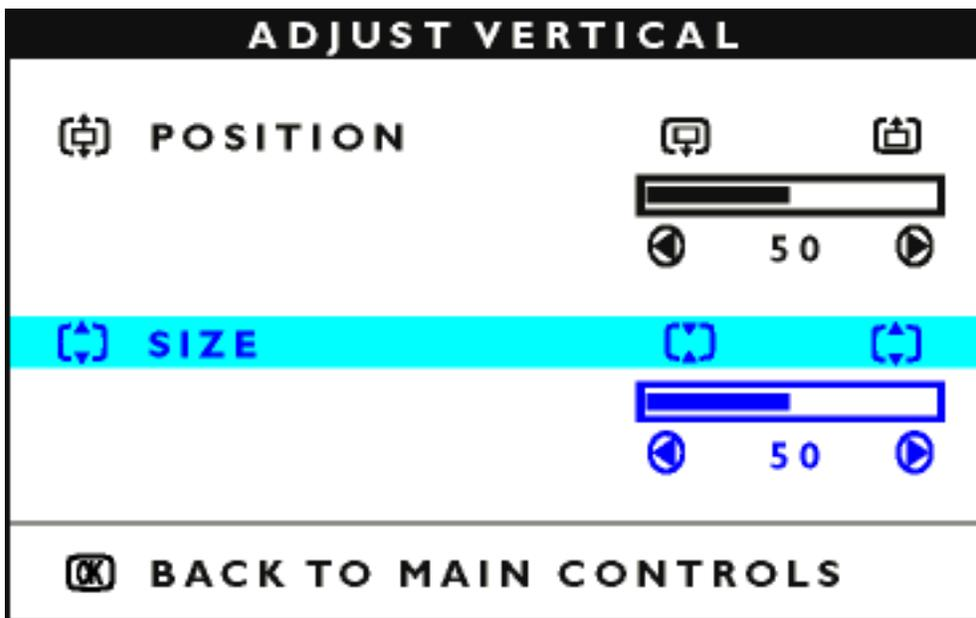
6) To adjust the vertical size, press the
