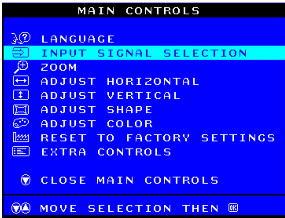
3) Press the
